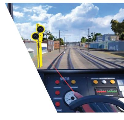
Trainees must deal with important scenarios. For example, in one module they encounter a shopping trolley on the track and must take appropriate action. This is exactly the sort of situation that was extremely difficult to prepare drivers for before the advent of VR.
